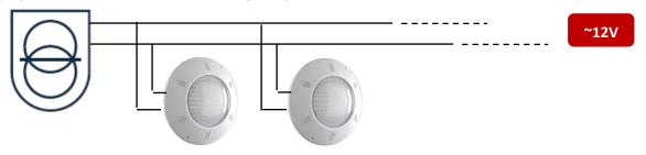
A N'UTILISER QU'AVEC UN TRANSFORMATEUR ISOLANT DE SECURITE. NE PAS BRANCHER EN SERIE. PROTEGER LES CONNECTEURS AVEC DU GEL ISOLANT.
